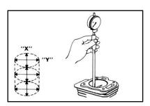
Cylinder Taper and Out of Round Specifications
