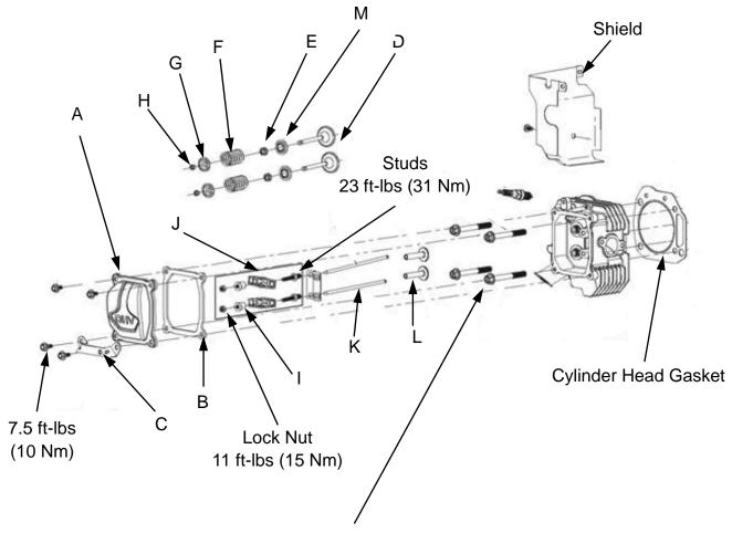
**Cylinder Head Bolt Torque Sequence:**
